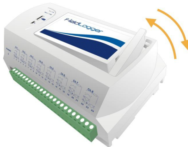
Fig. 09 – Attaching and detaching FieldLogger front cover
