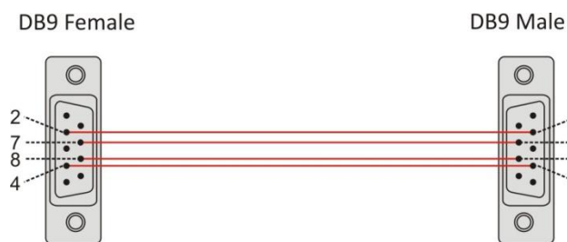
Figure 27 – Building an extension cable
